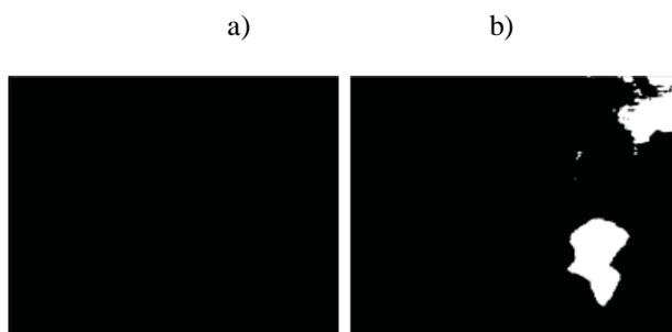
**Figure 6** a) Magenta color of thermographic image of commutator of healthy DC motor after binarization for  $T = 0.1$ , b) Magenta color of thermographic image of commutator of shorted DC motor after binarization for  $T = 0.1$
