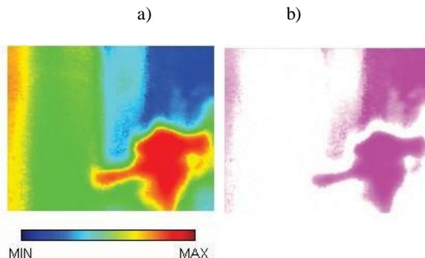
**Figure 5** a) Thermographic image of commutator of shorted DC motor,
