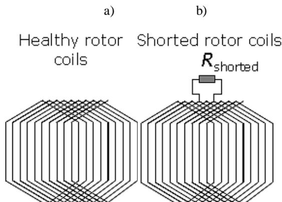
**Figure 9** a) Scheme of rotor windings of healthy DC motor, b) Scheme of rotor windings of DC motor with 3 shorted rotor coils
